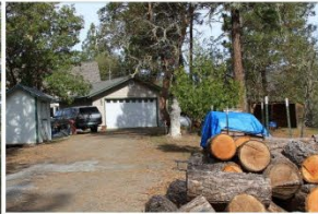
Store piles of lumber and firewood at least 20 feet from your home or other structures.
